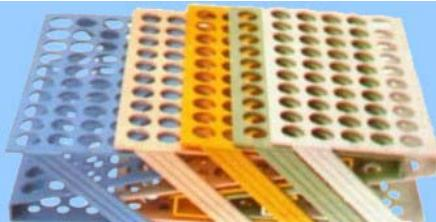
New Z - Form racks save space - over 55% reduction for storage. Manufactured from ABS material and are heat resistant up to 90°C. The alphanumeric marking allows for easy sample identification.
